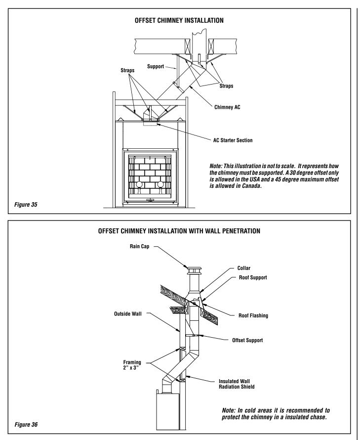
IF THE CEILING IS 9 FEET OR LESS THIS INSTALLATION CAN ONLY BE ACHIEVED USING 45° ELBOWS. SINCE ONLY 30° ELBOWS ARE ALLOWED. IN THE U.S. THE OFFSET MUST BE DONE ABOVE THE CEILING.
